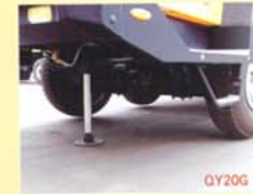
第五支腿 5TH JACK 扩展了起重作业的空间和范围, 大大提高了臂方区的起重能力。 Extend the space and range of lifting operation, and improve the lifting load capacity over front area.
